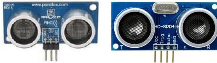
Gambar 2. Sensor ultrasonic
